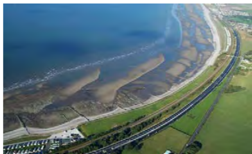
BROADENED SANDY COASTAL ZONE: SAND-ENGINE FOR COASTAL PROTECTION, UK ( HTTPS://PHYS.ORG/NEWS/2015-10-SAND-ENGINE-COASTAL-EROSION.HTML )
