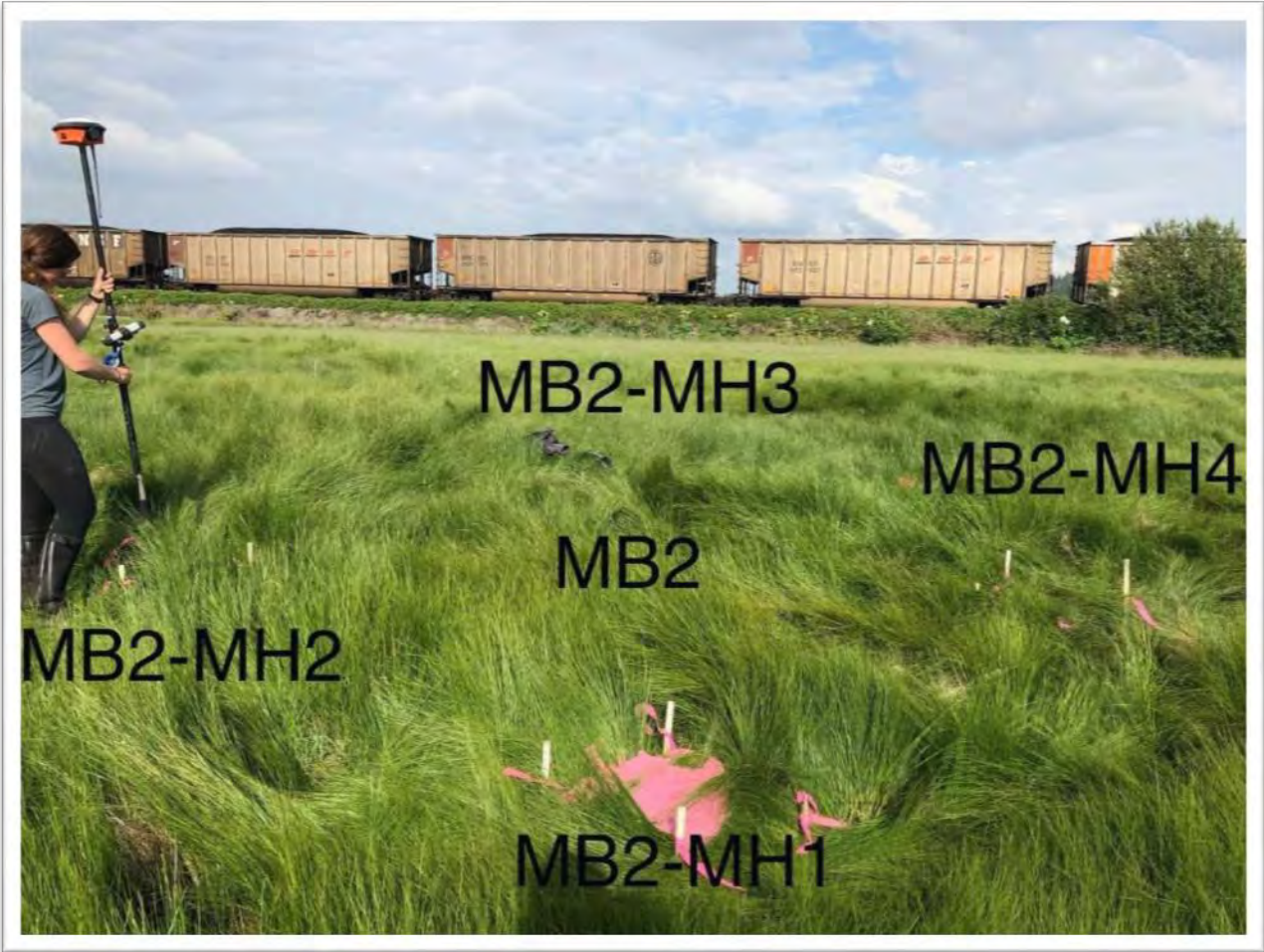
Figure 4 rSET platform (center) with four marker horizons approximately 3 meters apart
